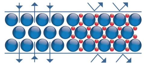
When viewed under a microscope, the particles in a normal roof membrane appear as they do on the left of this diagram, with small spaces between all particles. Adding smaller nano-particles fills these spaces creating a much stronger barrier to the elements.
